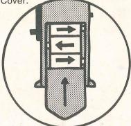
Some batteries vary in length. If unit does not operate, bend the battery contacts toward the batteries to assure proper contact.
