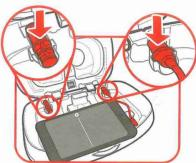
Insert the connector into your smartphone. Insert the other end of the cable into the space shown.
