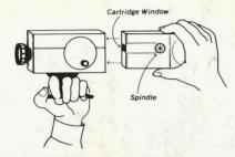
LOAD IT. Hold Action Viewer and cartridge as shown (cartridge window to left, spindle toward you).
